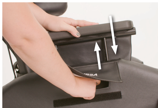
WHILE SQUEEZING lower or raise arm support
